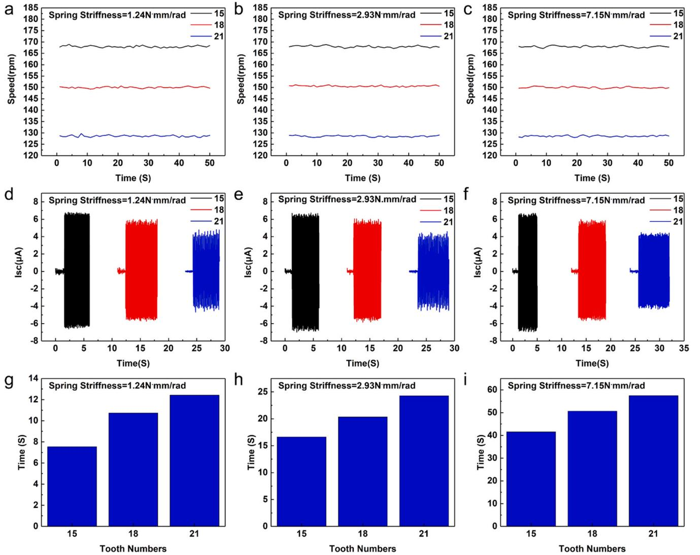
**Fig. 2.** Rotor speed, running time, and short-circuit current of the CO-TENG under fixed excitation conditions. Top row: Rotor speed under different numbers of ratchet teeth and same spiral spring stiffness; Middle row: Short-circuit current response to different numbers of ratchet teeth and same spiral spring stiffness; Bottom row: Running time on different numbers of ratchet teeth and same spiral spring stiffness.
