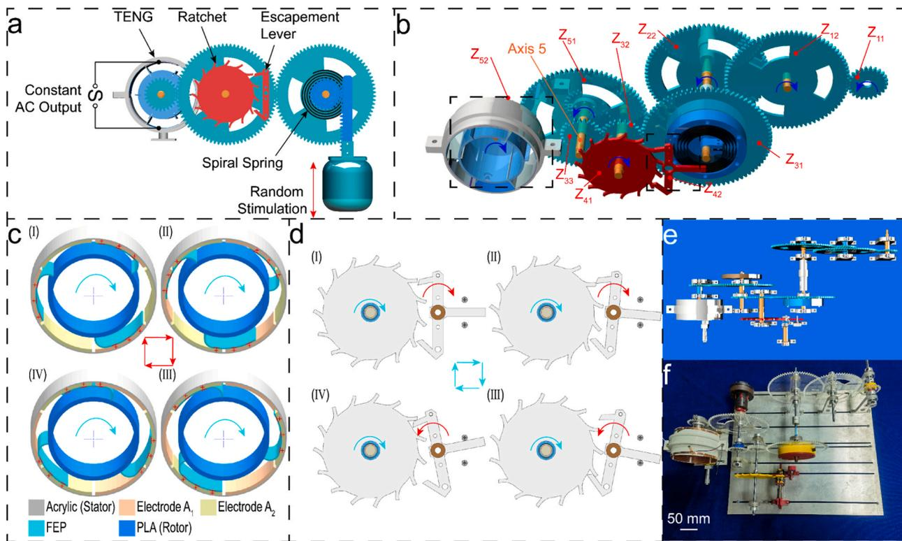
Fig. 1. Structure and working principle of the CO-TENG. (a) Working principle of CO-TENG; (b) motion transfer process of CO-TENG; (c) electric energy conversion processes; (d) operating principle of the escapement-spring-leaf mechanism; (e) floor plan of CO-TENG; (f) picture of whole structure of CO-TENG.
